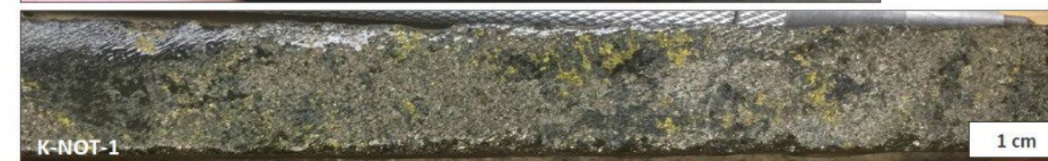
Massive sulfide mineralization with nickeliferous pyrrhotite and chalcopyrite
