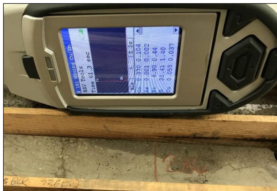
Drill core – Ni sulphides 4.90% Ni, 0.07% Co, 0.06% Cu
