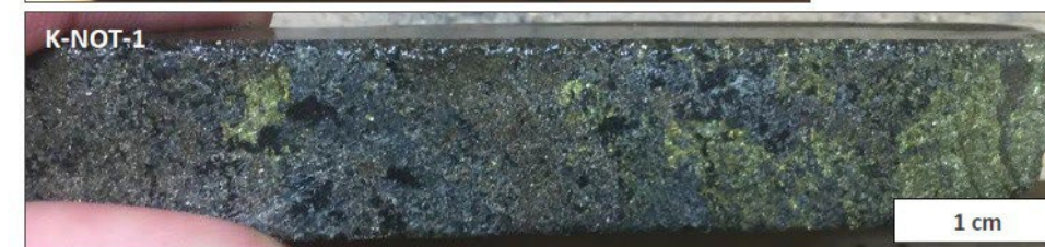
Massive sulfide mineralization with nickeliferous pyrrhotite and chalcopyrite
