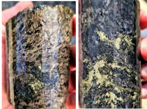
Figure 1: Vuostok Project (Storbodsund) massive sulphides: 3%-5% pyrrhotite, 0.5% pentlandite, 1%-2% chalcopyrite. From 5.7m to 7.2m in drillhole VUO23012
